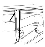
Diagram 3: Store the locking pin under the ramp
